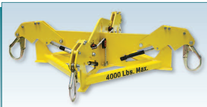
A Bag Lifting Rack for placing a bulk bag into an Acrison Bulk Bag Unloader with a hoist. The Lifting Rack (as shown) includes both Acrison's optional Automatic Bag Tensioner and Bag Liner Tensioner.
