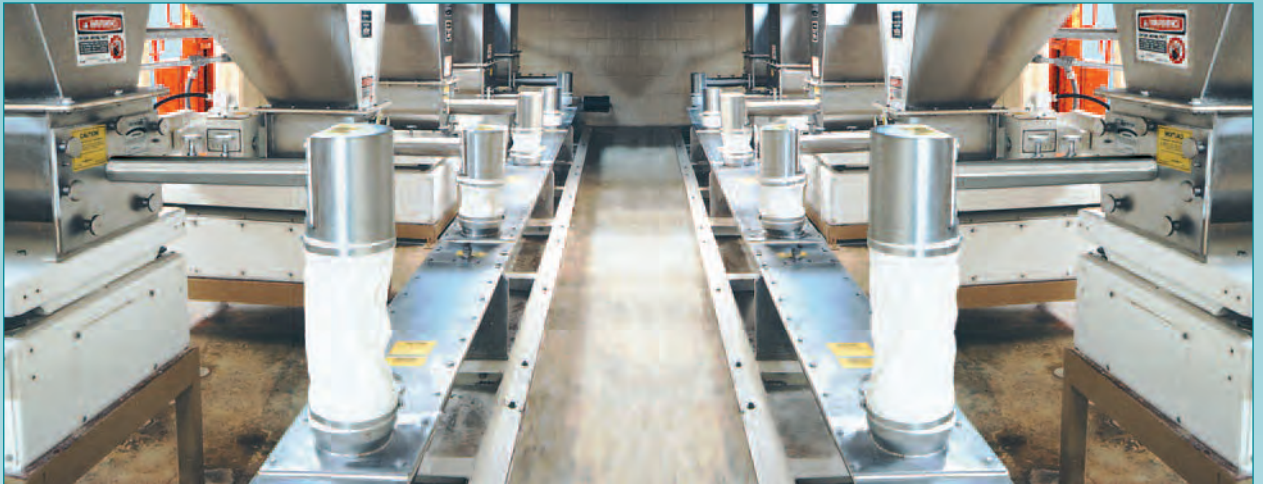
Two Model 301 Blending Systems incorporating a number of Acrison 'Weight-Loss' Weigh Feeders.
