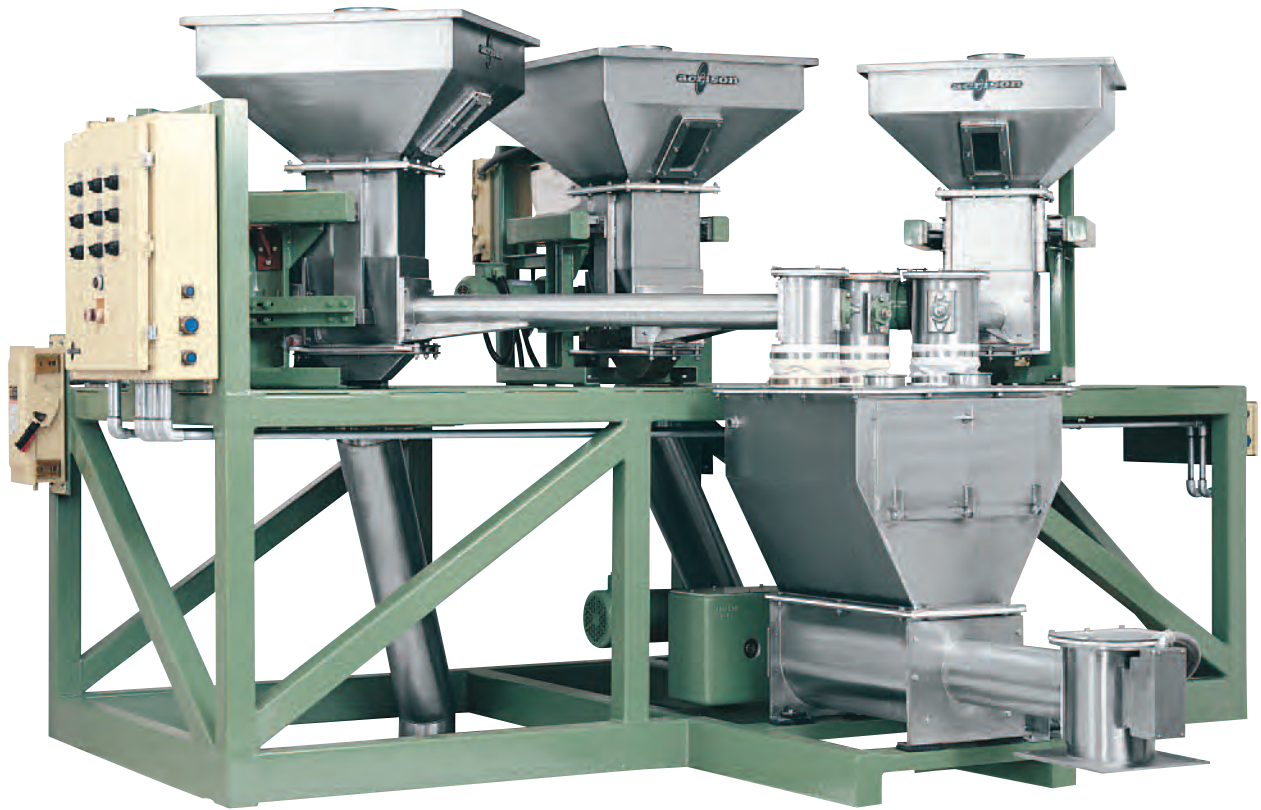
An integral Model 350 Blending System incorporating three Acrison 'Weight-Loss' Weigh Feeders.
