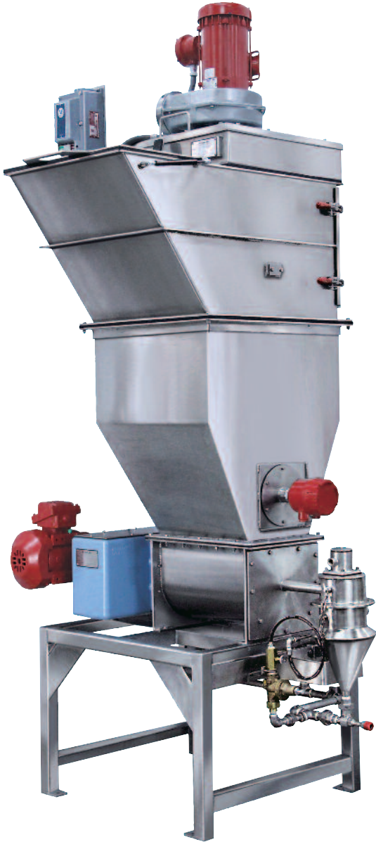
An Acrison Model DCBDS-400 (Dust Collector Bag Dump Station) mounted onto the hopper of a Model W-105Z Volumetric Feeder; the hopper includes a Low Level Probe. The Feeder is configured to meter a chemical into a Low Capacity Wetting Cone.
