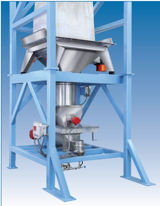
A Model 810 Bulk Bag Unloader discharging into the hopper of an Acrison Model 105Z Volumetric Feeder. A Maintenance Gate is provided above the Feeder's inlet. The Feeder is configured to meter a chemical into a Low Capacity Wetting Cone.
