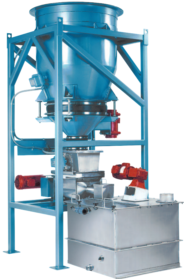
A Model W-105Z Volumetric Feeder mounted beneath a 50 cubic foot Storage Bin equipped with a Vibrating Bin Discharger. A Low Level Probe in the Feeder's Supply Hopper controls operation of the Bin Discharger. The Feeder is configured to meter a chemical into an Acrison 200 gallon Dissolving Tank.
