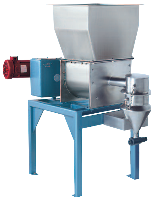
Volumetric Feeder with Wetting Cone Swirling water vortex and eductor mixing action ensure a consistent slurry discharge.
