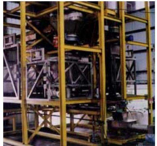
The 5-ton staging "mini-silos" feed raw materials into loss-in-weight feeders. Each of the mini-silos has a vibrating bin activator and a 12-in, knife gate valve. A 20-ft blender empties into another horizontal blender.
