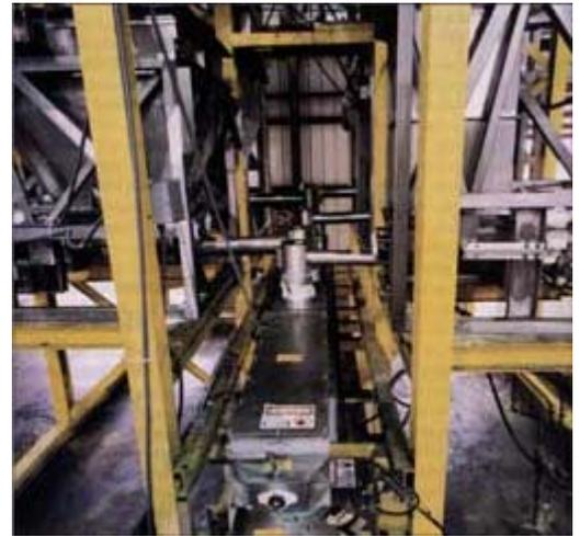
**Five loss-in-weight feeders meter raw materials into a 20-ft continuous ribbon blender, providing a constant product composition for packaging.**
