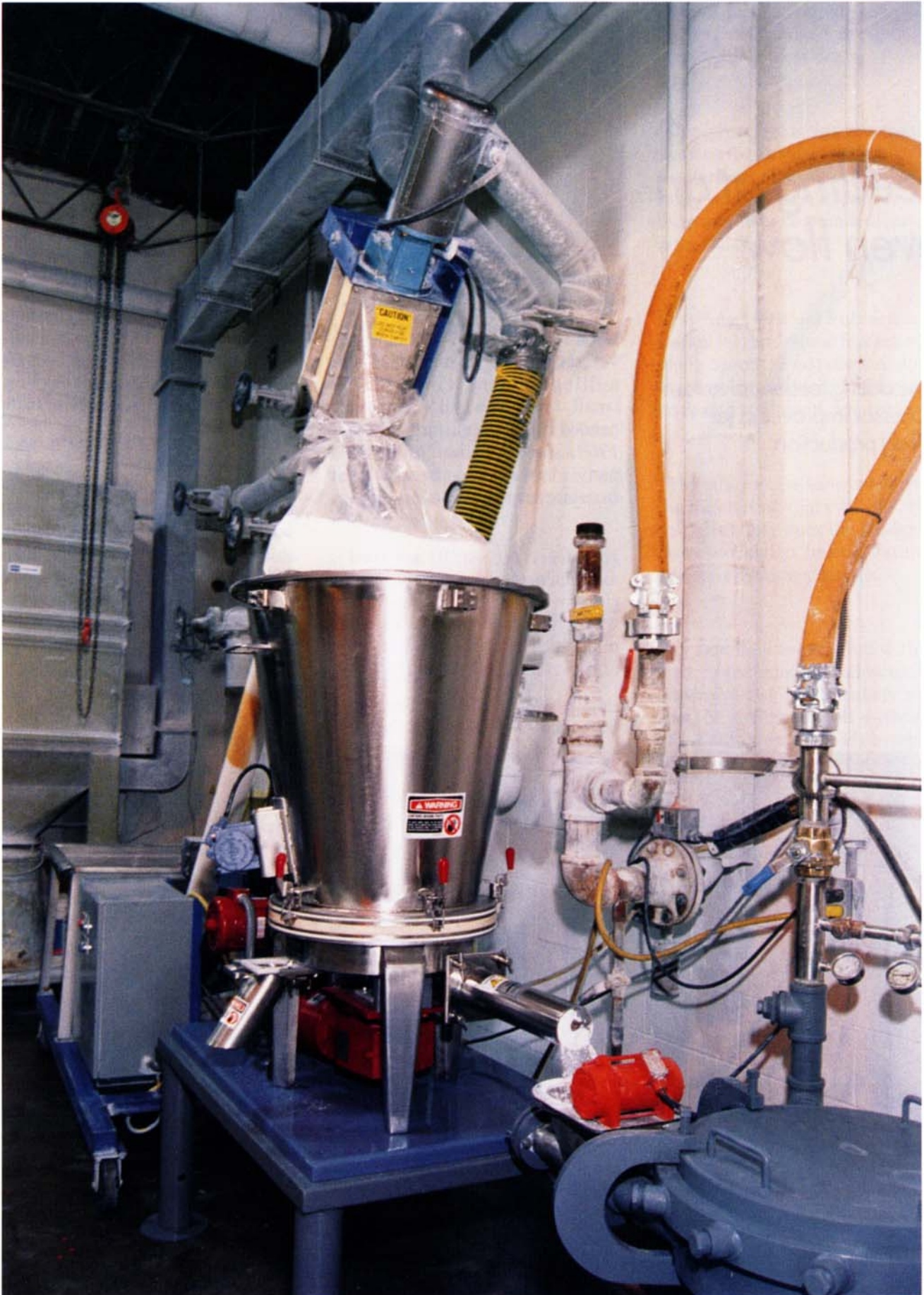
These feeders, with features such as a flat-bottom feed chamber and conditioning agitator, evenly meter hard-to-handle materials.
