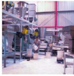
'We were keen to buy a feeder with two dissimilar feed screws, and particularly liked the Acrison version, as it has just one drive mechanism, making installation and maintenance easier.'
