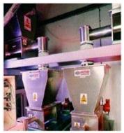
The feeders are remotely controlled via two MD-II-2000 controllers (located in the
