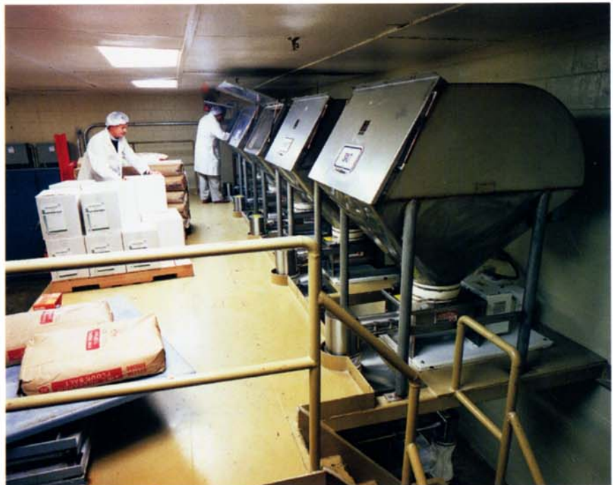
Workers empty dry peanut butter ingredients into bag-break stations positioned above volumetric refill feeders for automated feeding and blending.
