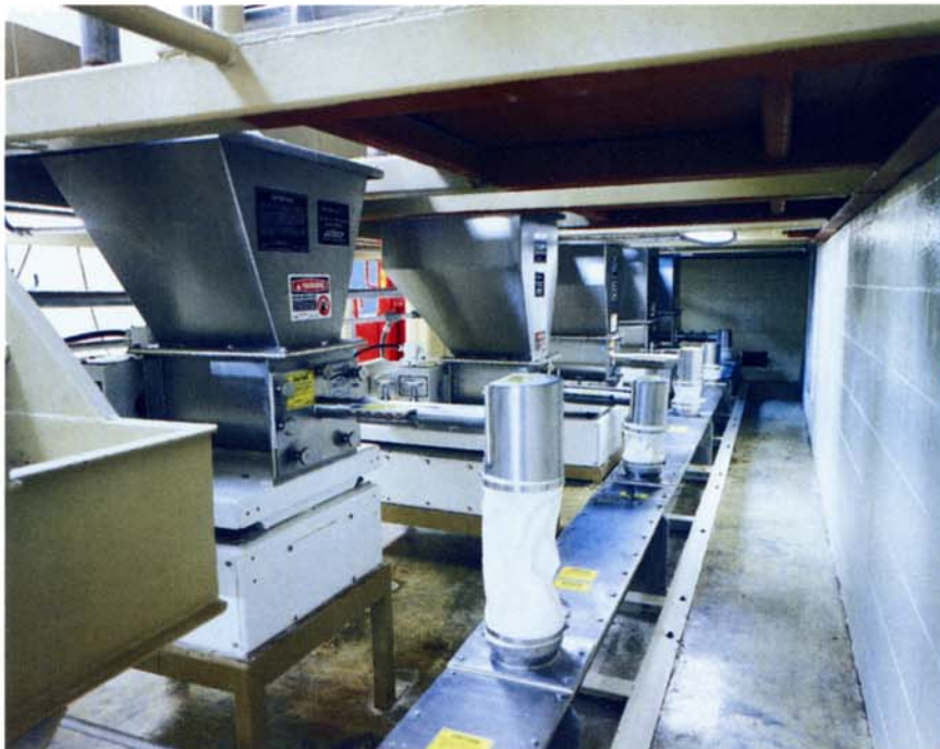
Loss-in-weight feeders meter the peanut butter ingredients to an auger preceding a blender that combines the ingredients before milling.
