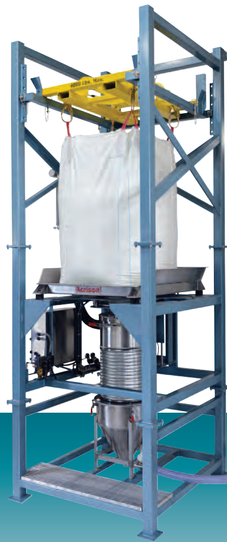
A Model 820 Bulk Bag Unloader discharging (on demand) into a pneumatic conveying system. The Bulk Bag is loaded by a forktruck, and the Bag Lifting Rack includes Acrison's optional Automatic Bag Tensioner.
