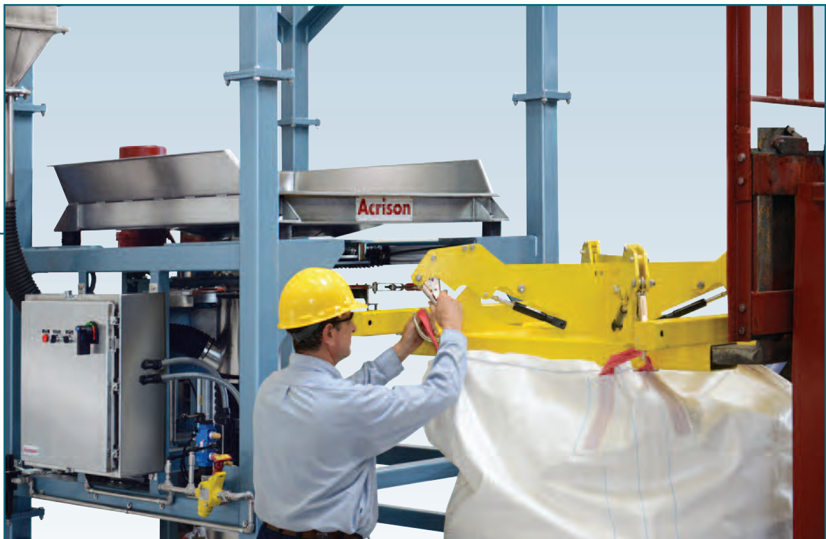
Operator attaching the lifting straps of a Bulk Bag to the Unloader's Bag Lifting Rack for loading by a forklift. The Bag Lifting Rack includes Acrison's Automatic Bag Tensioner.
