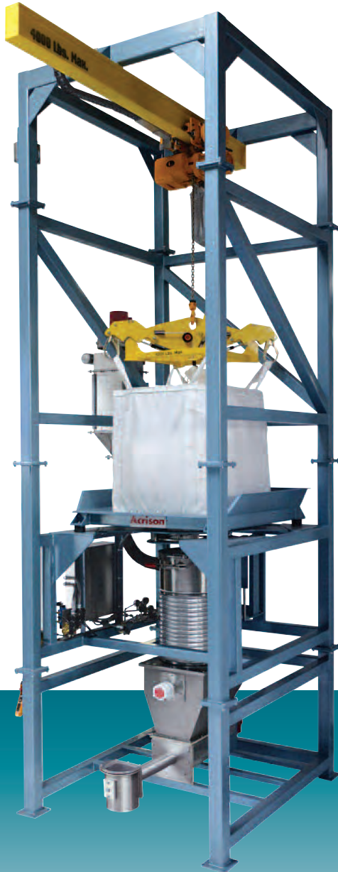
A Model 820 Bulk Bag Unloader discharging into an Acrison Volumetric Feeder (operates on demand by a level probe in the feeder's hopper). The Bulk Bag is loaded by an integral hoist and the Bag Lifting Rack includes both Acrison's optional Automatic Bag Tensioner and Bag Liner Tensioner.
