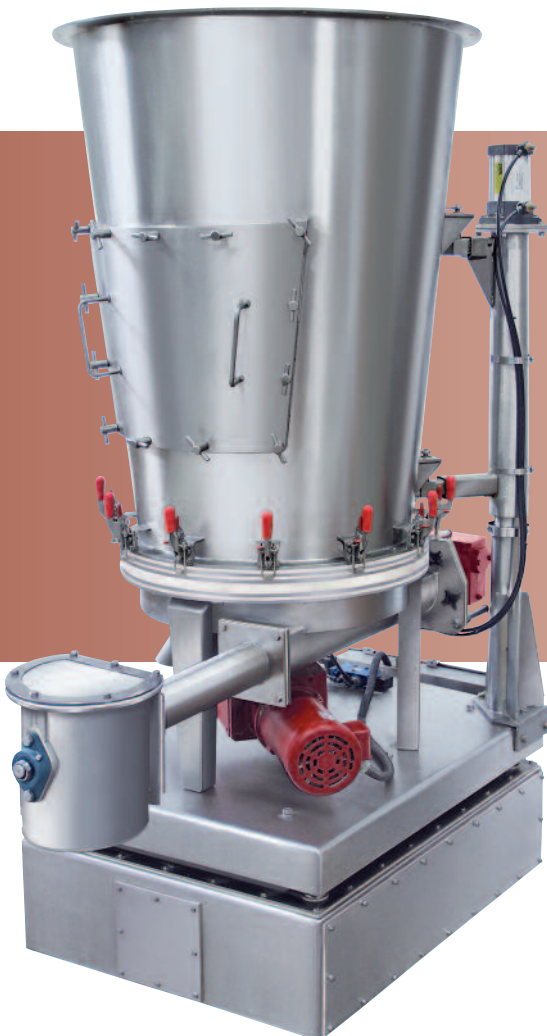
Model 402X-170-2 (Equipped with an optional hopper lift-off/swing-out mechanism, pneumatically operated)
