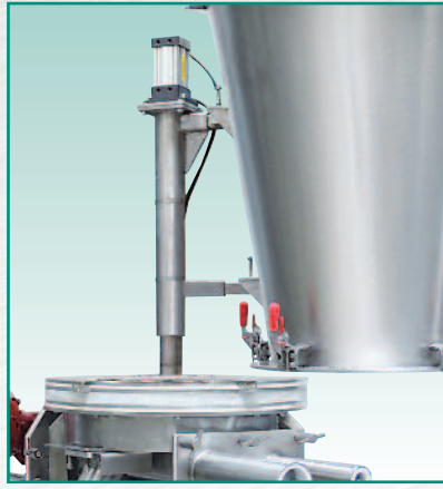
Pneumatically operated Swing-Out Hopper (certain models)
