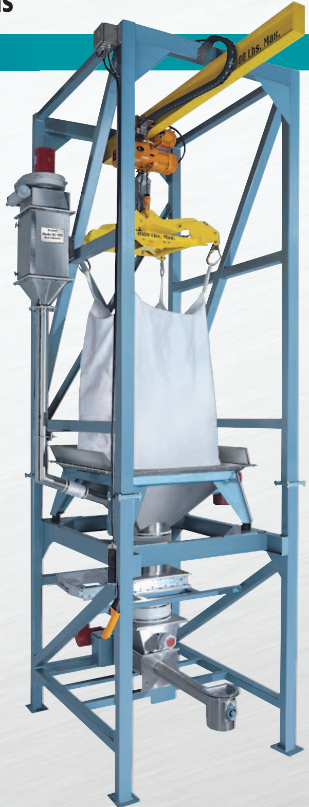
A Model 810 Bulk Bag Unloader mounted above an Acrison Volumetric Feeder (a maintenance gate is provided between the Bulk Bag Unloader and the feeder). This Bulk Bag Unloader includes an electric hoist and motorized trolley, Acrison's Automatic Tensioning Bag Lifting Rack, and a Dust Collector.
